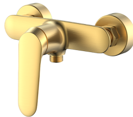
2501DES35-04SGD Shower Faucet Materials: Brass, Stainless steel Ceramic cartridge: dia.35mm Finish: Chrome, Matt black, Gun metal, Gold, etc
